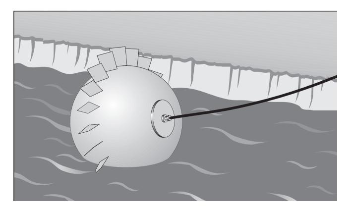
The PHEPP makes electrical energy from movement energy in the same way as a bicycle dynamo (see Figure 2). The movement of the water pushes against blades on the outside of the PHEPP and turns it while the inside stays still held by a weight.
